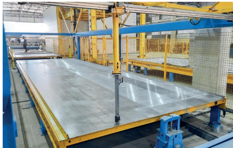
The plotter marks out the contours of the future concrete component on the pallet with precision.
