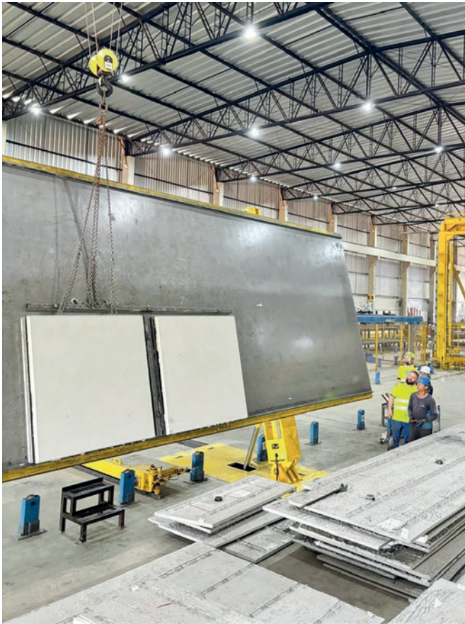
After production, the double wall elements are erected using the tilting mechanism, removed by crane and transported to their intended installation location.
