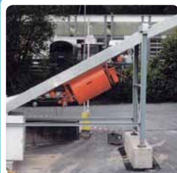
Rollover bucket in a 32° inclination = 60%
