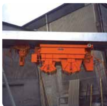
Double chamber bucket 3.000 / 1.500 l
